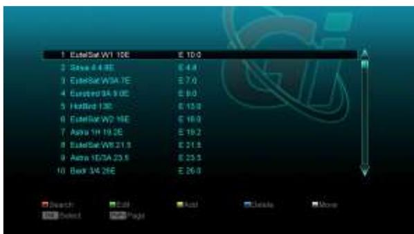
1. You can press [ok] button to select one or more satellites and press [red] button. it will show up a dialog to ask you scan mode, program type, scan type and NIT Search on/off. After you set up, press [OK] key to start
