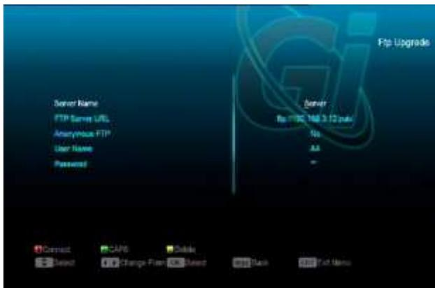
When connected to the Internet, receiver can make software update from file from FTP server.
