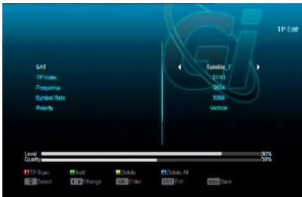
1 In “Satellite” item, press[Volume Up/ Volume Down]key to switch satellite that you want to scan or press[OK]key to enter satellite list for selection.
