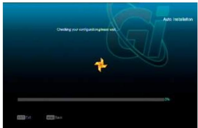
“Auto Installation” is a very new and convenient function. It will automatically detect all dishes connecting to this stb and scan the available services belonging to the satellite matched according to satellites and transponders data in current database. You don't have to input any parameter of your antenna settings. Just press “**OK**” button to enter this “Auto Installation” menu then it starts scanning and shows you the result at the end of scanning.
