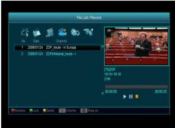
In this menu you can playback the record files, and you can press [Red] key to rename the file, or press [Green] key to lock the file, or press [Yellow] key to delete the file. You can press [1] key to adjust the volume while you preview the record file on top of the right corner .and you can press to enable or disable the audio.
