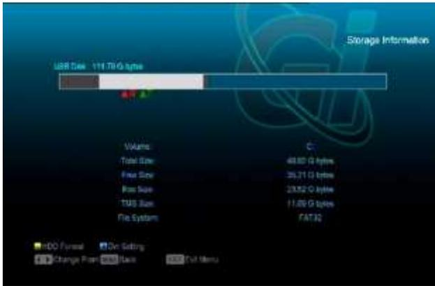
If you want to format the HDD, press "yellow" button to enter Format menu, then select the File System between the "FAT" and the "NTFS", Press "OK" Button to confirm.
