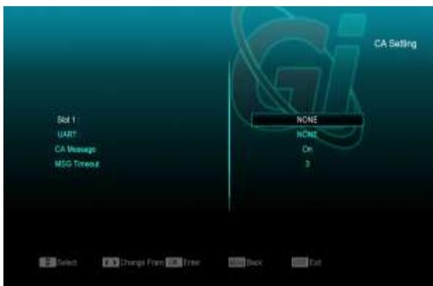
*Note: All information showed in this menu and submenu are coming from inserted card. In case if anything is wrong, it could be card problem. After inserting the card correctly at any time, a message-box will show on the screen with message about detecting the card, in "card info" menu all available information will be displayed. You can press [left/right] key to setting the message display time.*
