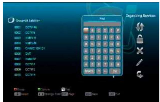
1. Press[Find] key can open the "Find" window like above. You can press[Channel Up/Channel Down/Volume Up/Volume Down]key to move highlight and press [OK] key to input the selected symbol or letter into the dialogue.
