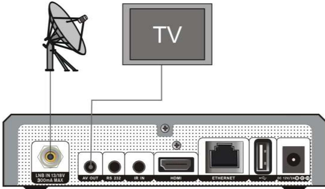
Finally connect the coaxial cable from the LNB to the LNB IN jack on the receiver.
