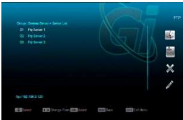
When connected to the Internet, receiver can download some files, such as software, MP3 or Image files from FTP server.
