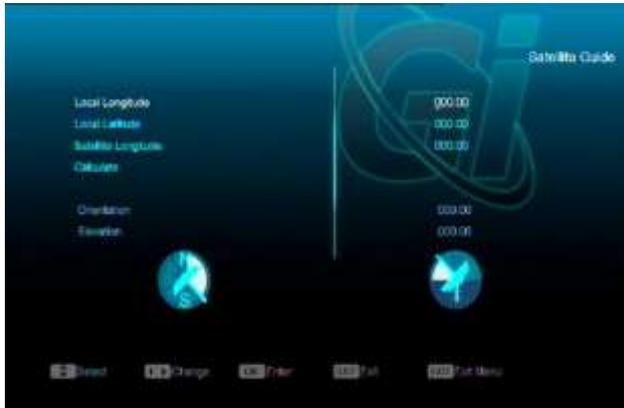
“Satellite Guide” is use for user to enter local longitude; local latitude and satellite longitude. By the evaluation from the receiver evaluate the antenna azimuth and antenna elevation; user can follow this guidance to adjust antenna.
