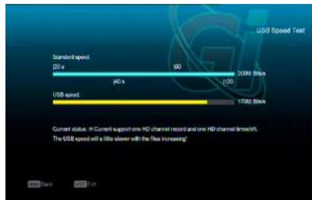
In "USB Speed Test" Menu you can see the Standard speed and your USB hard disk speed, according this information you can know what operation your disk can support.
